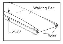
damaged. Using the allen wrench, turn both rear roller adjustment bolts counterclockwise 1/4 of a turn. When the tension of the walking belt is correct, you should be able to lift each side of the walking belt 2 to 3 inches. Walk on the treadmill for a few minutes. Repeat until the walking belt is properly tightened. Be careful to keep the walking belt centered.
